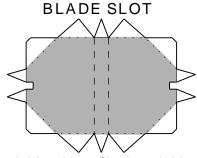
Cut a toothpick to 1" long. Glue the toothpick through the blade assembly and place into the cutouts of the blade slot. Glue inside chassis.
